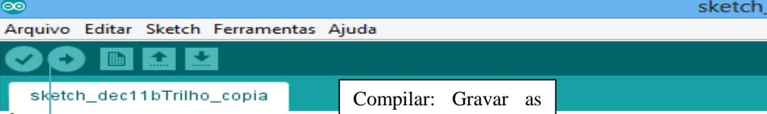
The image shows the Arduino IDE interface. The menu bar includes 'Arquivo', 'Editar', 'Sketch', 'Ferramentas', and 'Ajuda'. The toolbar contains icons for check, run, upload, and download. A callout box with a black border and white background points to the compile button (a right-pointing arrow) and contains the text 'Compilar: Gravar as informações na placa'. The code editor shows the following text:
