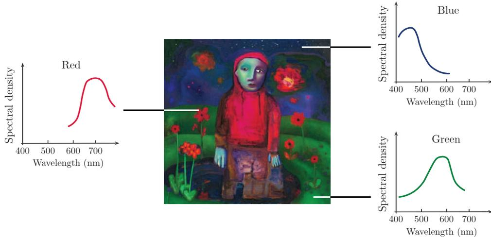
Figure 8 – Free representation of the spectral density as a function of wavelength at three positions in a color image. Adapted from figure 10.1-4 of [7]. In the image, the official album cover for the 2021 album 'If I could Make It Go Quiet' by Norwegian musician Girl in Red is utilized to illustrate how the spectral density translates to the perceived color.
