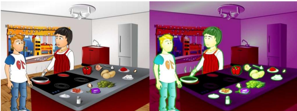
Figure 22 - Left: Standard visualization of a game scene from eAdventure game 'Eating Out'. Right: Adapted visualization of the scene for people with low vision. High contrast rendering mode is applied darkening the background and highlighting the interactive elements
