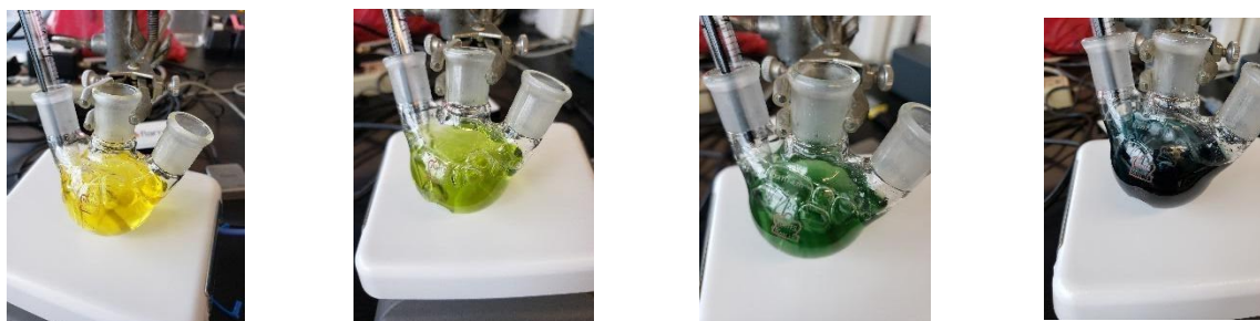
Figure 7 - Oxidation of 1,1- ferrocenedimethanol (yellow) to its oxidized form (blue)
