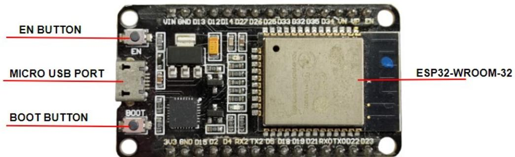
Figura 3.4: NodeMCU-32S com microcontrolador ESP32-WROOM-32.
