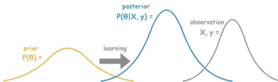
Figure 3.2: Learning process through Bayes' rule. A new observation is used to update a prior probability distribution yielding a new posterior distribution.
