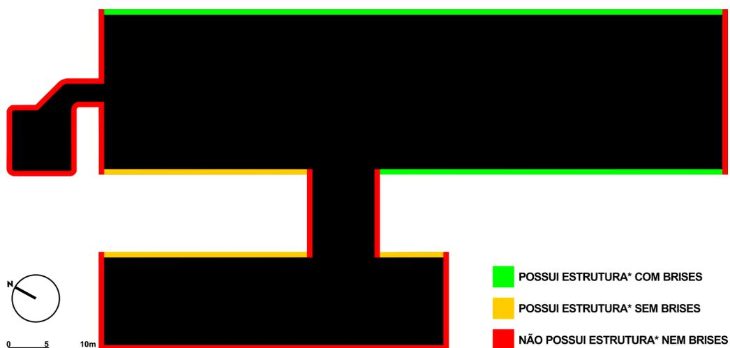
\*ESTRUTURA DE PILARES E VIGAS QUE DISTAM, APROXIMADAMENTE, 40CM DA FACE EXTERNA DA FACHADA, FORMANDO UMA ESPÉCIE DE MOLDURA PARA COMPORTAR OS BRISES VERTICAIS.
