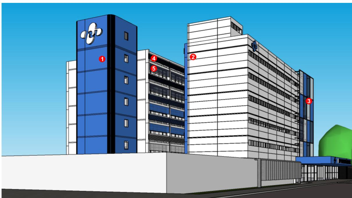
1: ACM AZUL; 2: ACM BRANCO GELO; 3: PAINEL DE MEMBRANA TÊXTIL VERTICAL; 4: BRISE HORIZONTAL; 5: PAINEL DE M. T. HORIZONTAL.
