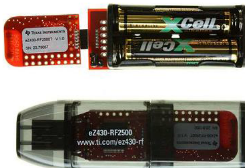
Figura 3.1: kit eZ430RF2500 da Texas Instrument's (TEXAS-INSTRUMENTS, 2011a).
