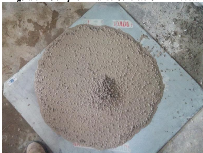
Figura 61 - Slumpflow final do Concreto CARMR5060.
