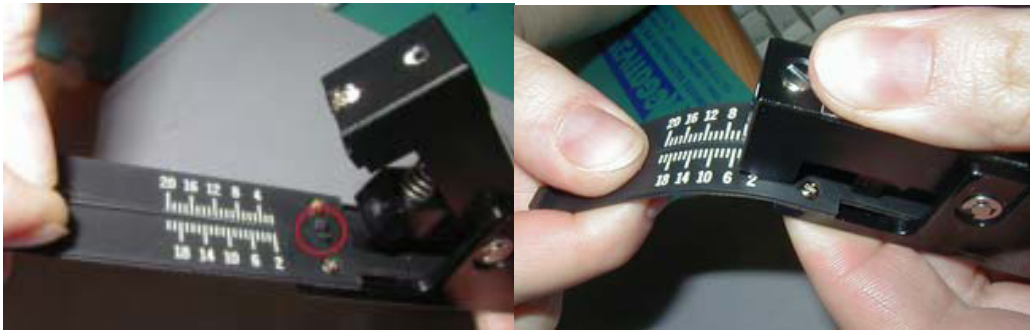
(a) Posicionar a fibra no cleaver.
