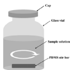
Fig. 2. Schematic of SBSE set-up.
